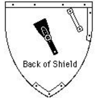
Depiction of handle placement on a heater-style shield.
